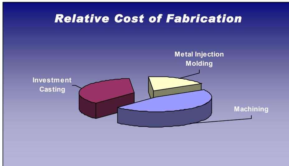
The more complex the part, the more cost effective metal injection molding (MIM) becomes. The cost savings can be substantial, often as high as 25-70%.
